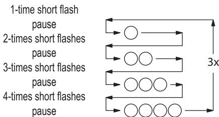
The flash sequence will repeat 3 times and start with 1 short flash. If no confirmation is given, by pressing the
