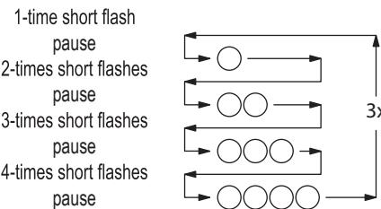
The flash sequence will repeat 3 times and start with 1 short flash. If no confirmation is given, by pressing the
